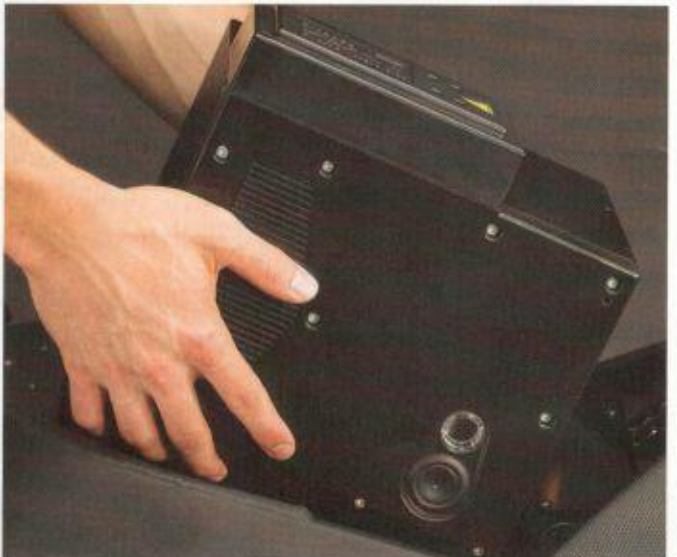
The S and DS come with a "tank" bag, that sits in the empty space not occupied by a petrol tank. Otherwise, you can put a whole extra battery in there, increasing your range to as much as 276 km
