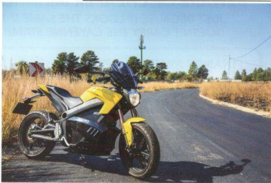
This is the Zero S, and it is far from the horrible eco-boxes that the car people go on about. Most of where the engine would normally be is battery, and the engine sits where the swingarm joins the frame.
