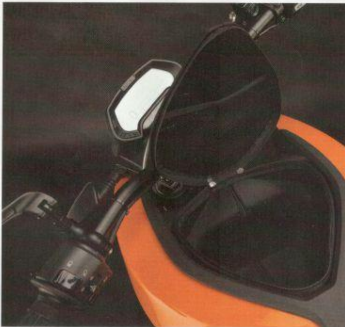
The S and DS come with a "tank" bag, that sits in the empty space not occupied by a petrol tank. Otherwise, you can put a whole extra battery in there, increasing your range to as much as 276 km
