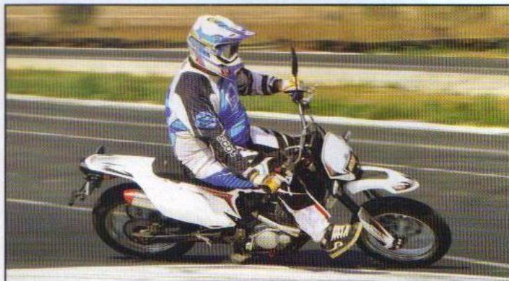
Designed as a motard, it has wide 'bars making it very easy to steer. The adjustable suspension and road tyres also help. Note the footpeg dragging on the ground.
